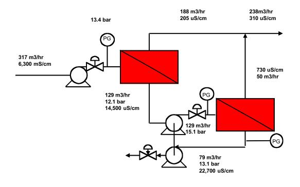
Flow diagram of a RO unit equipped with ESPA membrane elements at the Jupiter plant
